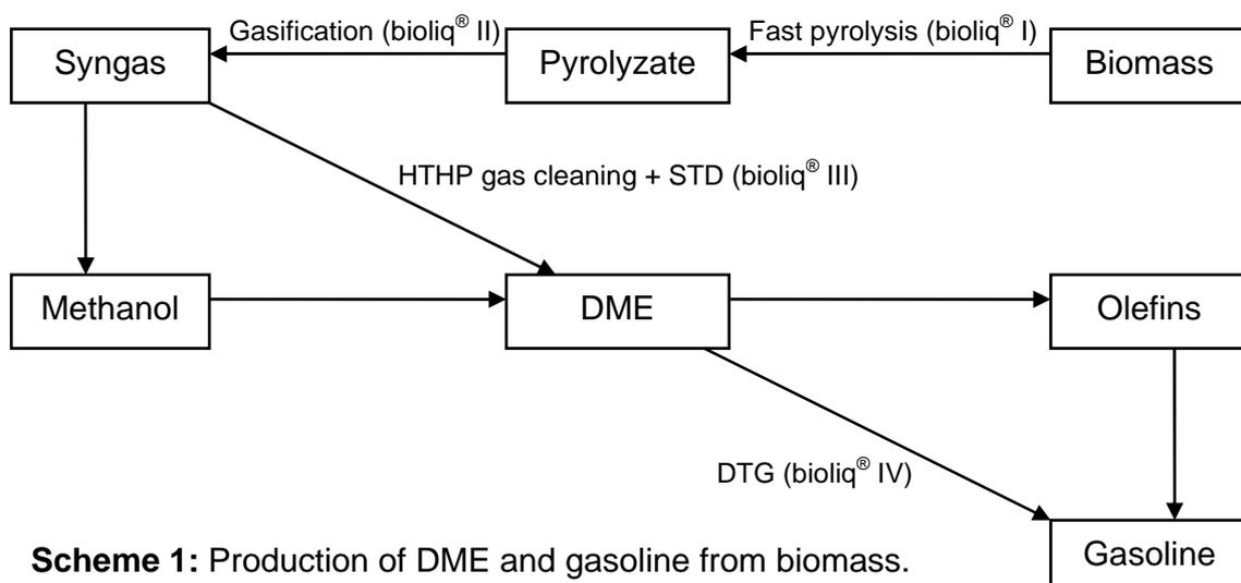
**Scheme 1:** Production of DME and gasoline from biomass.
